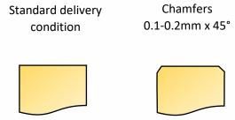
The chamfer add-on is applied on the electroded side and can be ordered at one or both ends of the plate actuator.
