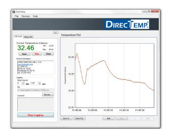
(Above) A screen capture of the DirecTemp interface, showing data plotting and logging options.
