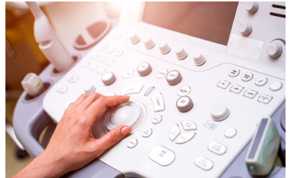
Ultrasound scanners often employ panel potentiometers to adjust display visuals.
